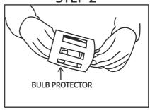
TAKE THE BULB PROTECTOR AND SETTLE BULB SOCKET WITH ELECTRICAL WIRE IN
