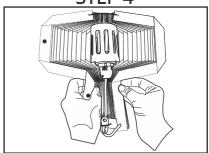
FIX THE SOCKET IN THE CENTER OF THE SHADE BY PLACING THE HOOK ON ELECTRICAL WIRE .
