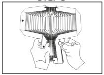
PUT THE WIRE IN THE CENTER OF THE RING AFTER OPENIG IT THEN CLOSE THE RING ONCE THE WIRE IS INSERTED.
